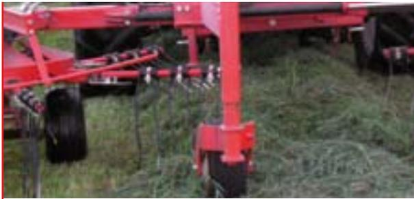
The optional front wheel is there to follow the contours on uneven ground resulting in cleaner raking and less wear and tear on the machine.
