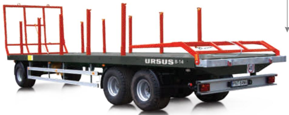
B-14 platform has a innovative security of frony and rear wall. In the design two lines inside the trailer were used. This solution provides protection against damage of foil of the bale. The high-resistant steel floor is consisting of a one single piece. The option included: toolbox 45 l, foldable side protection made of aluminum and stakes
