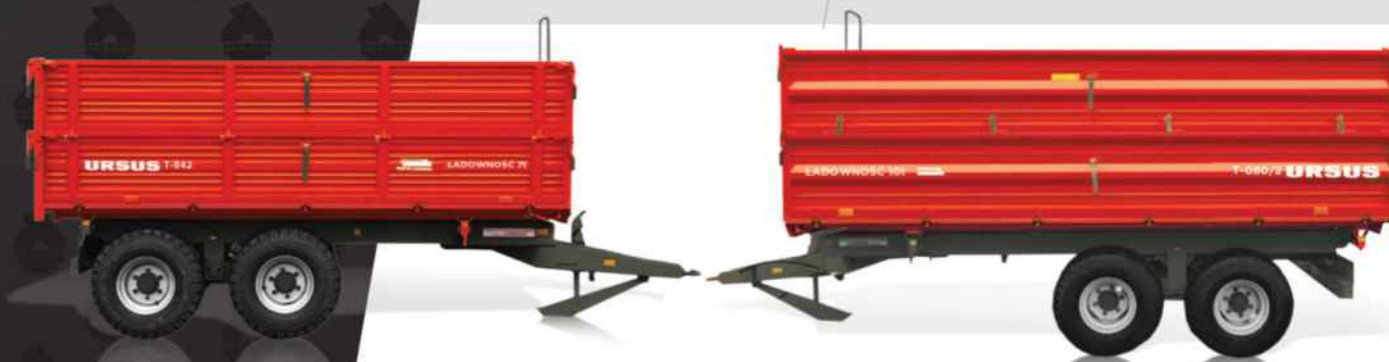
diameter of the drawbars eye 50mm [40mm in option]
