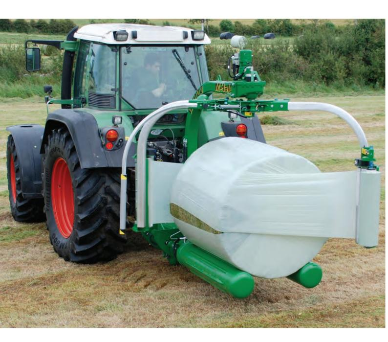
he McHale W2020 is a high-speed stacking bale wrapper. It is a compact machine, which allows one operator to transport, wrap and stack the bale with one tractor or loader. The W2020 can wrap a bale with four layers of plastic in approximately 20 seconds and with six layers of plastic in 30 seconds. The W2020 is controlled by an expert plus control box, which makes wrapper operation fully automatic.
