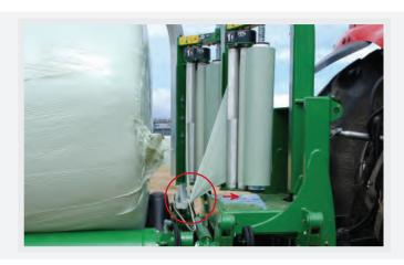
Automatic Film Break sensing comes as standard on the W2020 stacking round bale wrapper. This ensures that if one of the rolls of film breaks or runs out, the W2020 will detect this and slow bale rotation and increase the number of revolutions of the satellite to ensure that the bale is wrapped correctly. If both rolls of film break or run out the W2020 stacking round bale wrapper notifies the operator in the cab via the control box that the machine is out of film.
