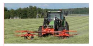
The cam operated rake arms ensure gentle raking into a well formed, fluffy and even swath. The swath width is hydraulically adjustable to make the optimal swath for the pick up on the following machine.
