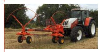
For road transport the rake is swung forward. The rotors, safety guards, and rake arms can be moved to their narrowest position to reduce transport width.
