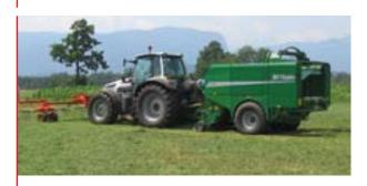
The purpose of the hydraulic driven front rake is to have a baler or loader wagon behind the tractor offering big savings on fuel, working hours and an additional tractor & driver.
