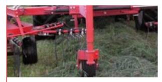
The optional front wheel is there to follow the contours on uneven ground resulting in cleaner raking and less wear and tear on the machine.
