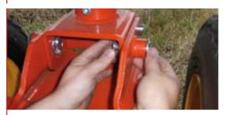
The ground wheels are adjustable for each rotor, which allows the rake to be adjusted for all field conditions. The wheels rotate 360° and operate independently.
