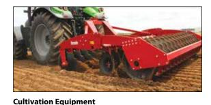
High performance tillage range including 'Multidisc' disc and tine combination harrows and 'Roterra' power harrows. Polymat pneumatic drills also available.
