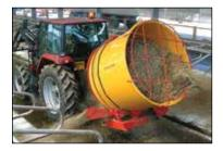
**Drum Mill System**Available with various screen sizes for chopping material to a consistent length, from 13mm to 125mm.
