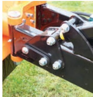
Collision protection in offset arms
