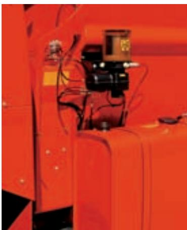
A new automatic greasing system, made of a pump with a 5 lt. reservoir, assures the periodic lubrication of all the bearings. This system can be operated even manually, by a lever in the cabin, if the greasing is required at different times.
