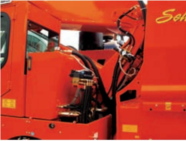
The hydraulic system consists of seven pumps. Two pumps with pistons and three with gears are assembled on the engine flywheel, and two more flanged pumps on the side PTO of the engine.
