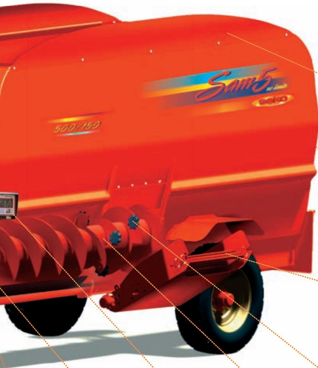
New upper edges for containing bulky fibrous products, with maximum shock resistance.
