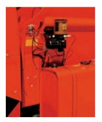
A new automatic greasing system, made of a pump with a 5 lt. reservoir, assures the periodic lubrication of all the bearings.
