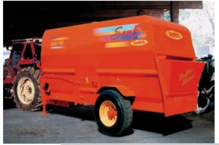
The rear hopper , of wide dimensions, allows an easy loading of the most different products in limited quantity, such as flour, mineral salts, integrators and additives.
