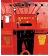
• Control console with "push-pull" lever controls
