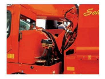
The hydraulic system consists of seven pumps. T pumps with pistons and three with gears are assembled on the engine flywheel, and two more flanged pumps on the side PTO of the engine.
