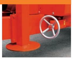
• Mechanical hand brake, applied by hand wheel
