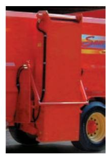
Side discharge through tilting conveyor available up to 3 m long
