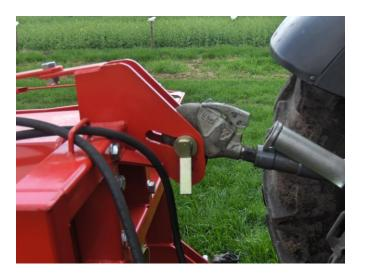
The top link attachment is equipped with two holes, and an oblong hole for working in lightly undulating terrain.
