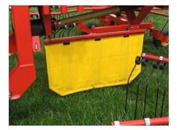
Strong and flexible shield between the rotors ensures that no material is flung from one rotor to the other, thereby ensuring an even and uniform swath.
