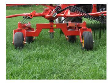
Strong and flexible wheel suspension with four large pivoting wheels, staggered to ensure optimal functioning and minimal wear on the machine.
