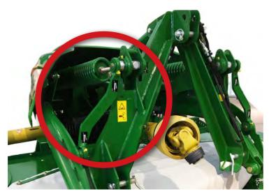
The McHale Pro Glide front mower range is fitted with patented active spring compensator technology which ensures that the mower cutter bar always applies the same ground pressure regardless of the working height.
