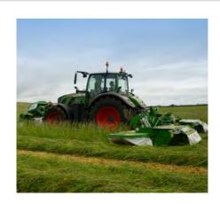
The Pro Glide range of rear mowers are fitted with patented ground adaption technology, which allows the bed to move back and up if the bed encounters small obstacles. This saves time and maximises throughput as it means the obstacle does not trigger the main break back protection. This results in higher mowing speeds being able to be achieved without the interruption of having to reset the break back.
