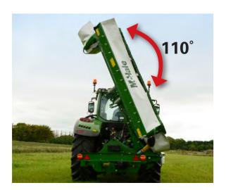
For transportation, the McHale Pro Glide folds vertically to position itself behind the centre point of the tractor for safe transport. The transport height of the machine is reduced as the mower bed is at 110 degree angle.
